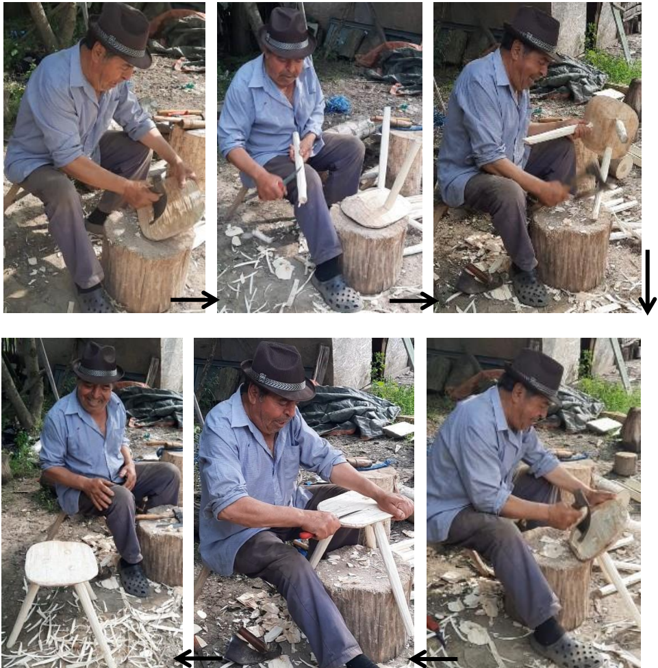
Fig. 2. The stages of making a three-legged chair
