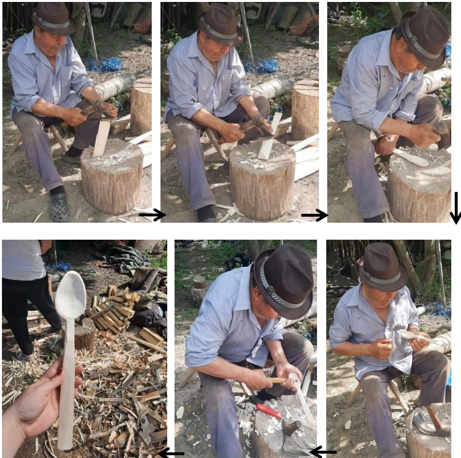
Fig. 3. The steps of making a wooden spoon
