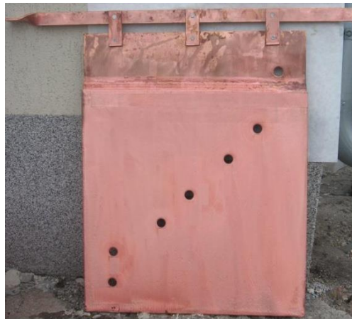
Figure 7: Cathode produced in laboratory L-SX-EW facilities
